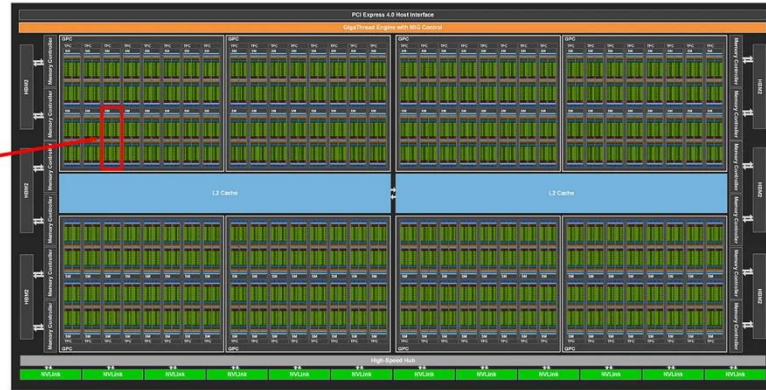
GA100 Full GPU with 128 SMs
